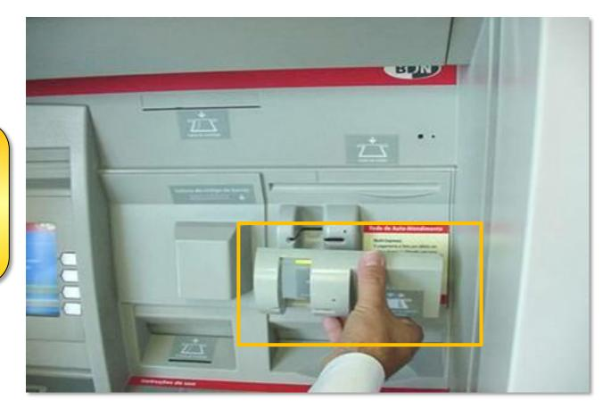
A skimming device being 'piggy-backed' onto the card reader
