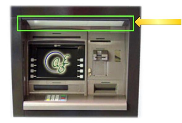
Photo shows a PIN capturing device fitted to the top of the ATM. These devices are usually difficult detect.
