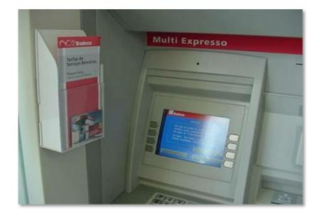
Take a closer look at the brochure holder – a pin-hole Camera has been installed. This is done to capture images of the keypad and customers inputting their PIN.
